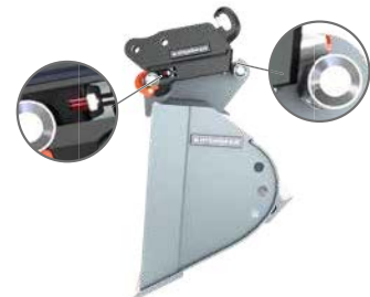
Not correctly locked. Locking pins are above the permitted range. Indicator pin is extended.
